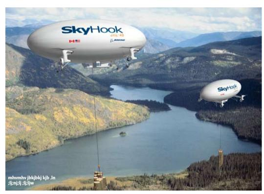
◄ The JHL-40, which will be developed and built by Boeing, combines a neutrally-buoyant semi-rigid helium envelope with four Chinook helicopter rotors. The inert gas provides enough lift to support the aircraft, leaving the rotors to lift cargo – 40t at a time – and propel it at up to 70 knots (130km/h) over its range of 320km.
